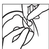
If required, to prevent gas from escaping, place one of the enclosed filter labels on the filter.
